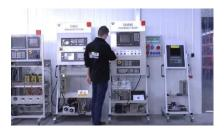
We have test stands developed by us, thanks to which we check whether the device is operational. They make sure that ALLEN BRADLEY 1333-AAB is repaired.
